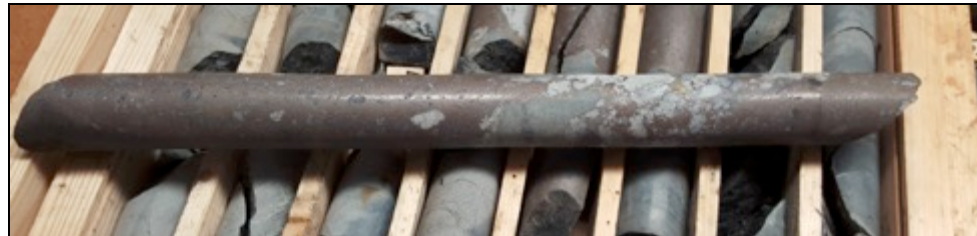
High grade zinc mineralization from Gumsberg in 2016 EMX DH GB16-2: 2.8 meters of 17.9% Zn, 6.9% Pb, 0.5% Cu, and 68.9 g/t Ag at a depth of 32 meters below surface. True widths are approximately 80-90% of reported drill intercept. (See Company news release dated September 8, 2016) B6
