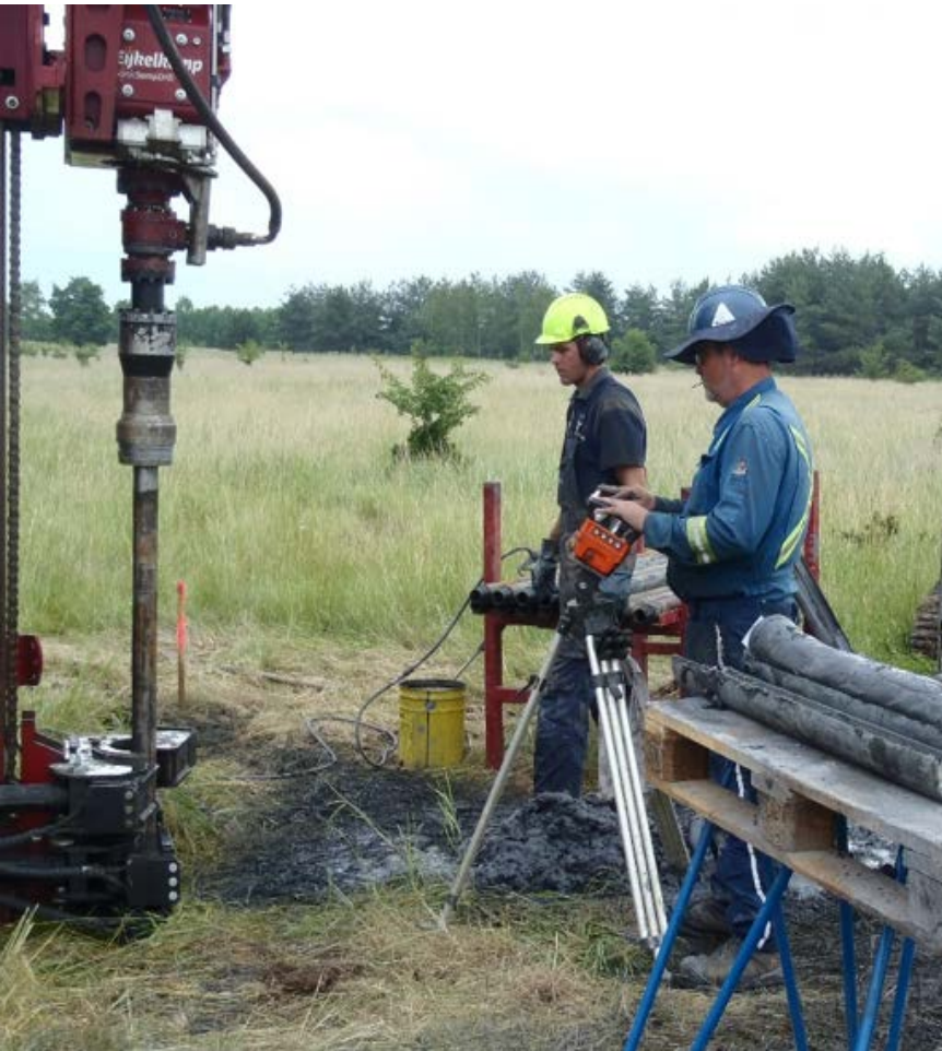
↑ Sonic drill – modern, effective sampling tool
