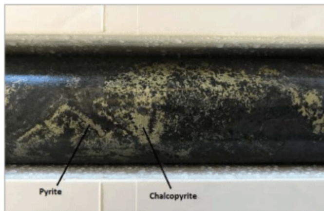
Figure 4. Interstitial chalcopryite mineralisation, diamond drill hole WND17-001 – 255.7m depth.
