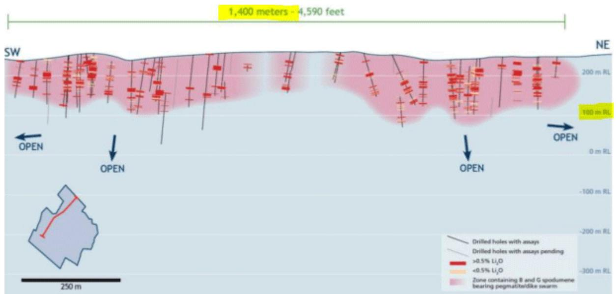
Figure 1: Piedmont Lithium Project – Schematic Northeast-Southwest Long Section
